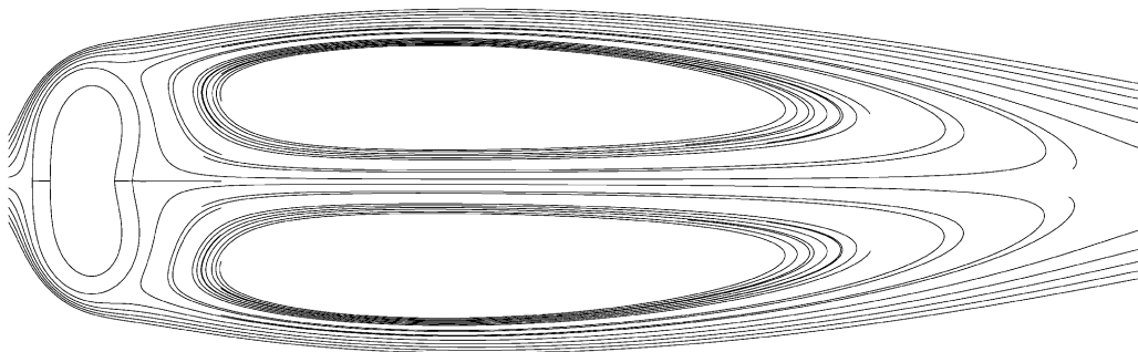
Fig. 10. Streamlines for the flexible cylinder a uniform flow.
